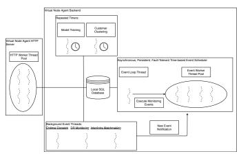
Fig. 4. Physical (implementation) diagram of our virtual node-based agent.
