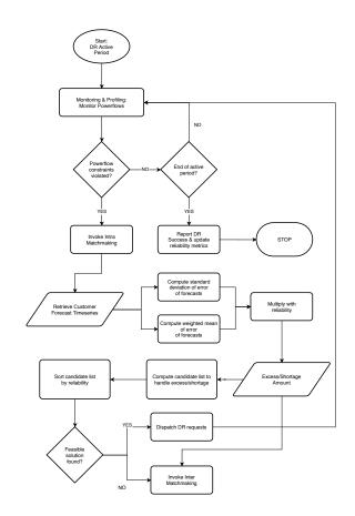
Fig. 2. Agent DR monitoring and Intra matchmaking flow diagram.
